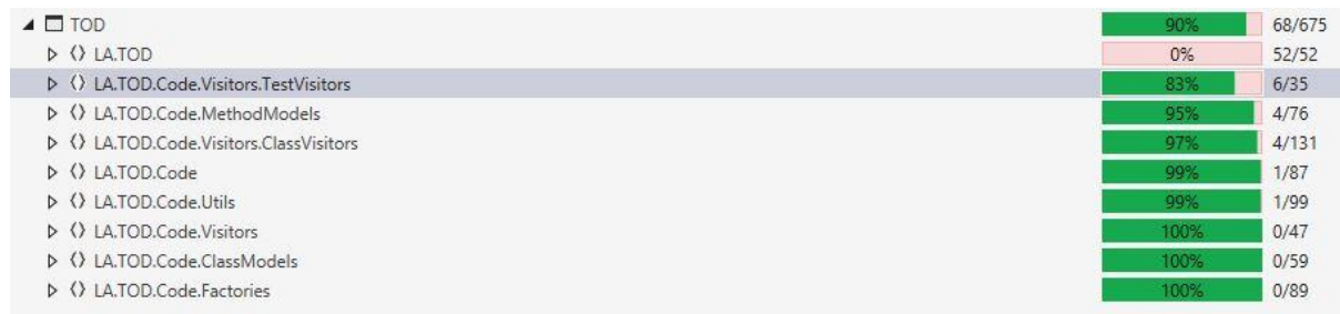
Figure 14: Test coverage of the TOD tool; the code in the root folder is the code provided when you create a package, hence it has no test coverage. The final column is the number of statements not covered by tests which adds up to 16/623 statements of my own code.
